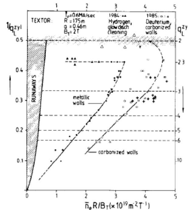
Fig. 8. Operational regime of TEXTOR with ohmic heating for conventionally RG-cleaned and for carbonized surface conditions [30].
