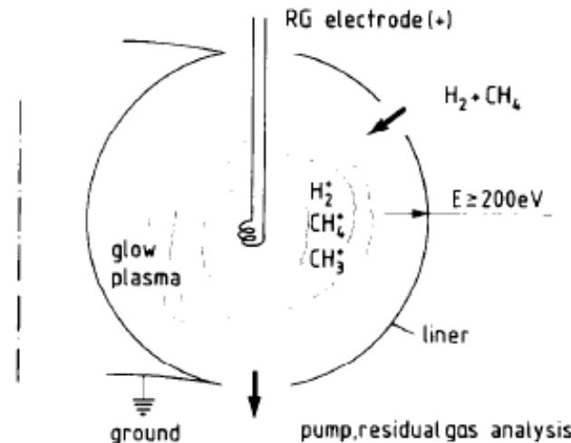
Fig. 1. Schematic sketch of the carbonization technique as developed at TEXTOR.
