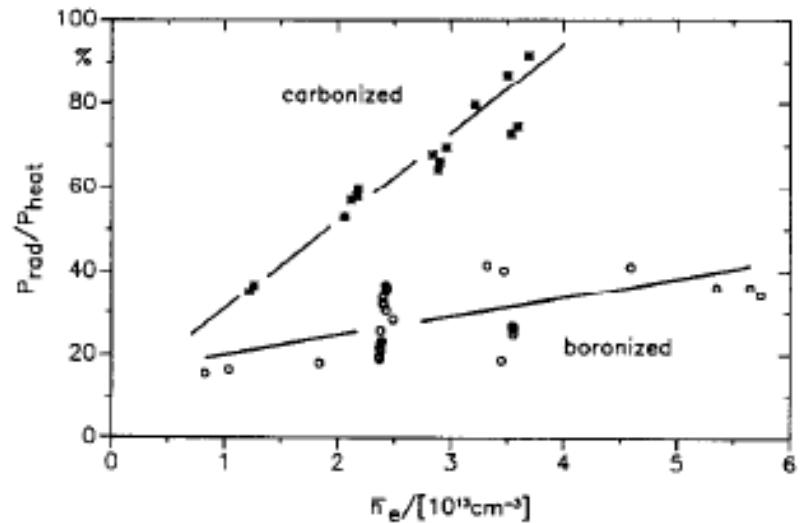
Fig. 7. Fraction of the radiated power  $P_{rad}$  relative to the ohmic input power  $P_{heat}$  for carbonized and boronized walls and limiters. Data for carbonized wall conditions have been taken from ref. [10].
