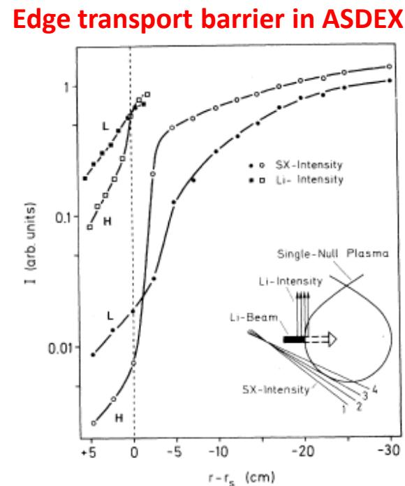
FIG. 2. Radial profiles of the SX (2- $\mu\text{m}$  Be filter) and Li-beam intensities in the L phase prior to the H transition and shortly afterwards (SX,  $\Delta t = 20 \text{ ms}$ ; Li,  $\Delta t = 55 \text{ ms}$ ).  $I_p = 375 \text{ kA}$ ,  $B_T = 2.2 \text{ T}$ ,  $\bar{n}_e = 3.3 \times 10^{13} \text{ cm}^{-3}$ ,  $P_{NI} = 0.8 \text{ MW}$ . The inset depicts the observation geometry.
