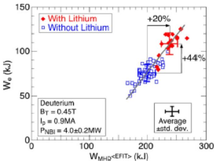
Fig. 3. Total stored energy from EFIT analysis and electron stored energy from volume integration of Thomson scattering measurements of  $n_e$ ,  $T_e$  for similar H-mode discharges with and without lithium coating of the lower divertor.
