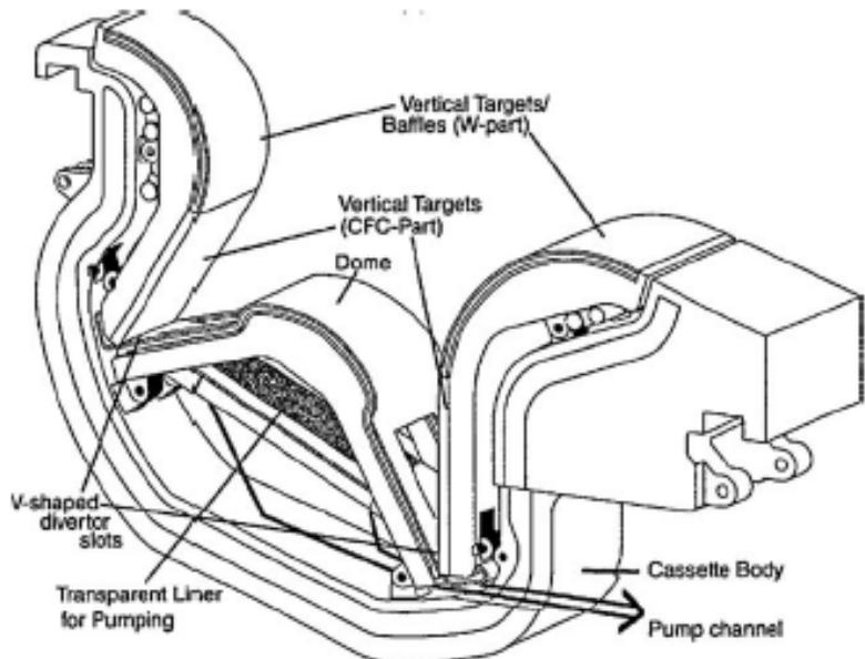
Fig. 5. ITER divertor design 2009 [3].
