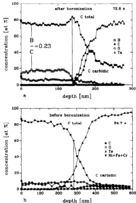
Fig. 2. AES depth profiles of redeposits collected at  $r \sim 46.7$  cm on the electron drift side Ta-targets after boronization (a) and before (b) when TEXTOR was carbonized.
