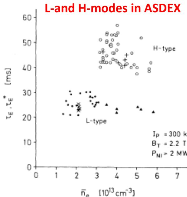
FIG. 2. Global energy confinement time vs average line density for toroidal limiter (triangles) and divertor discharges (other symbols).  $\tau_E$  (plusses and crosses) is deduced from thermal profiles and  $\tau_E^*$  (open circles, solid circles, and triangles) is determined from the diamagnetically measured  $\beta_{p\perp}$ .
