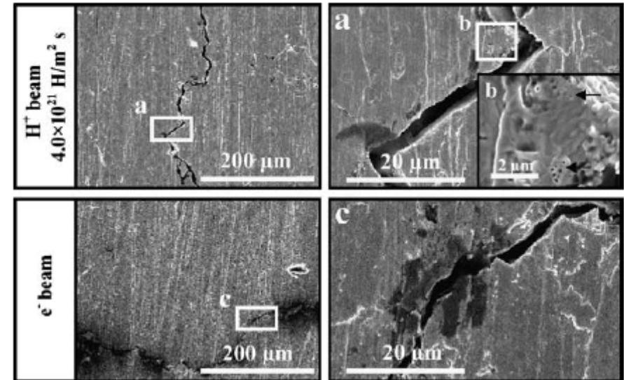
Tritium may be co-deposited into cracks.
