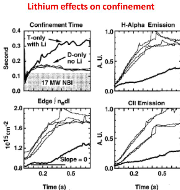
FIG. 6. Reduction in edge electron density and  $D\alpha$  and CII line emission and corresponding increase in energy confinement time for a T-only discharge (thick line) with good Li conditioning, and several D-only shots for comparison (thin lines).
